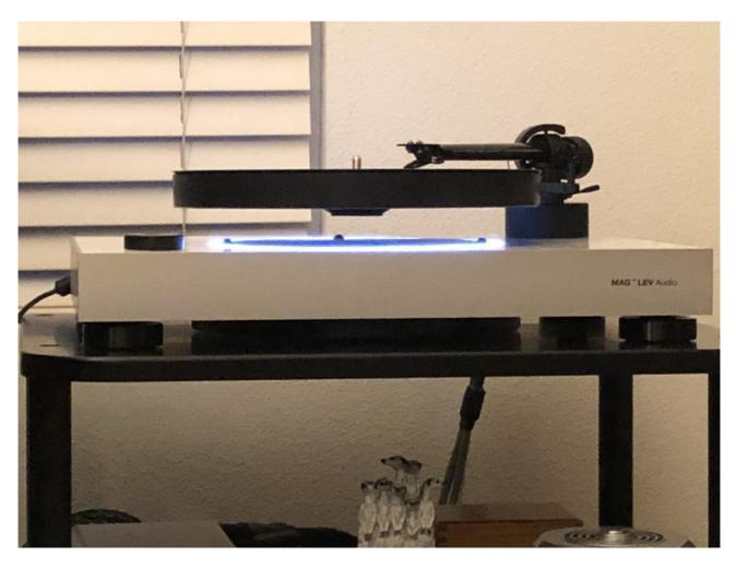
Wow and flutter...less than .17%. Weight is 9.8kg all in! Four sensors, two magnetic and two optical to maintain precise speed and stability. The ML1 is delivered beautifully packaged and pristine, with all tools and cables to perform like a breakthrough and super cool turntable should sound. As an audiophile of 55 years, I then turned it into GODZILLA!
